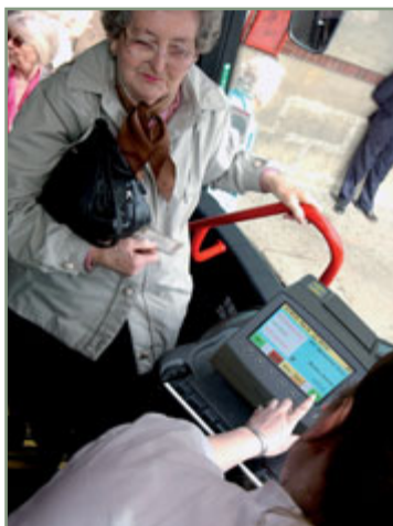
> EVENDsmart: Ticket printer and on-board computer in a single box.
