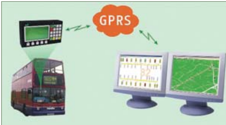
> The depot and the vehicles communicate via radio communication, based upon GPRS (General Packet Radio Service)
