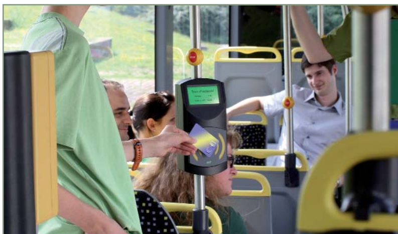
> The PROXmobil smart card reader allows passengers to utilize a check-in / check-out system and automatically calculate fare at the best rate.
